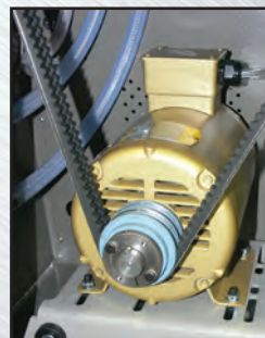
NEMA Premium® efficient inverter-driven motor
