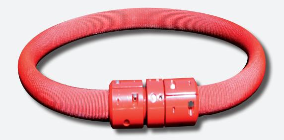
Scope: A multi-purpose, lightweight, rigid 1" diameter attack hose that meets the needs of industrial, municipal and forestry market applications. This uniquely constructed product features an all polyester cover for heat and abrasion resistance, along with a special helical interior reinforcement to retain its rigid shape. This thin-walled polyurethane lined hose, is the most durable lightweight booster hose on the market.
